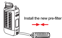
Figure 2: Installing the New Pre-filter
